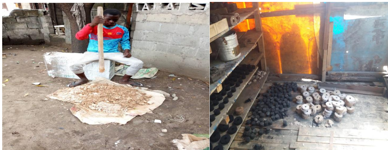
Briquettes making - left: preparing the waste and right: processed briquettes
